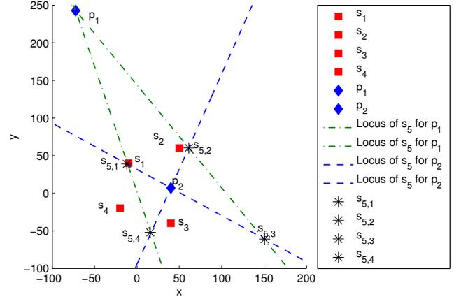
Fig. 1. Placing the fifth sensor at any of the positions indicated by \* results in an ambiguous solution for the position of the target.
