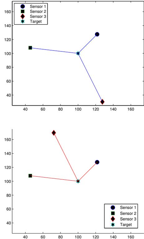
Fig. 2. This figure illustrates two scenarios obtained from each other by reflecting a particular sensor about the emitter position. This reflection does not affect the optimality of the sensor-target configuration.
