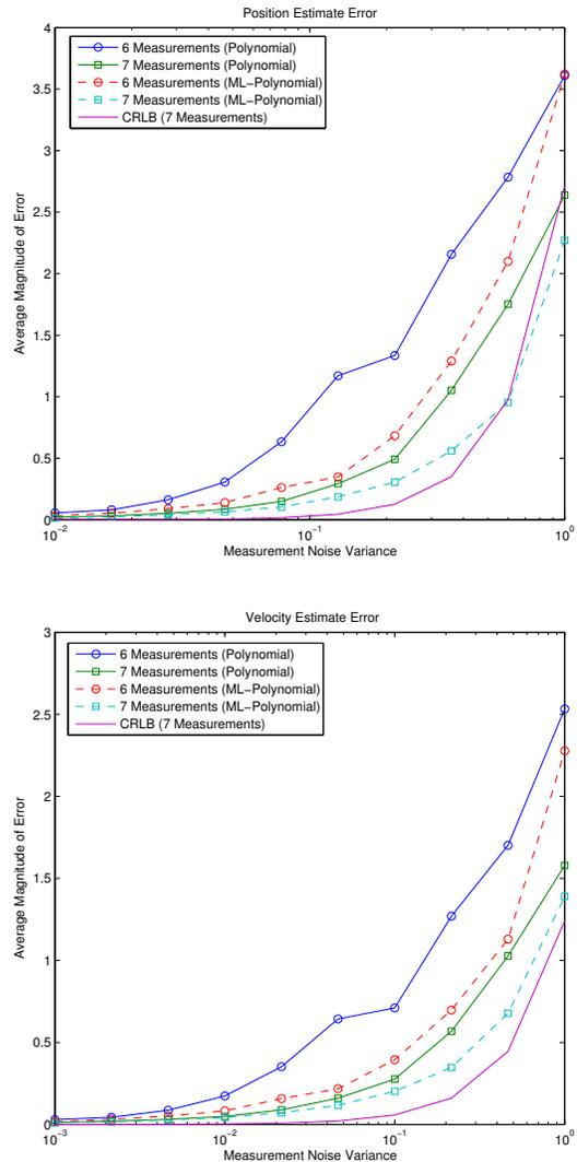
Fig. 4. The error in the estimate of the position and the velocity of the target using the proposed polynomial optimization method (Polynomial) and maximum likelihood initialized at the solution of the optimization problem (ML-Polynomial) after repeating the scenario 100 times with variable noise variances when six and seven sensors are used.
