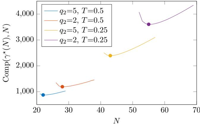
Fig. 2. Computational complexity over prediction horizon length for different system parameters.
